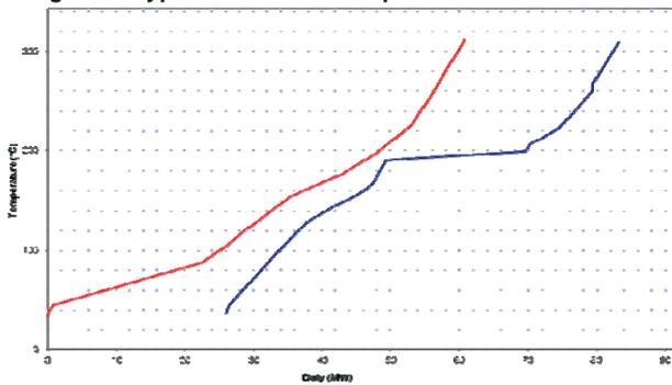
Figure 3: Typical Prime G+ Grand Composite Curve
